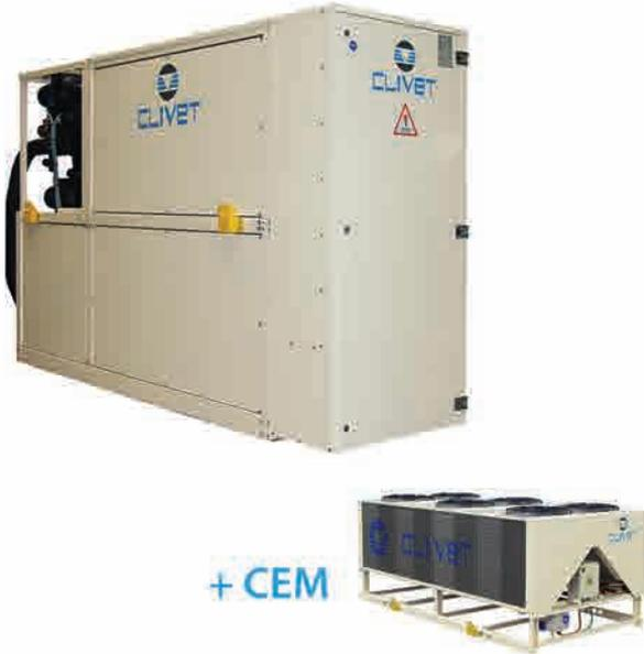
The **MSE-SC** units belong to the **SPINchiller** family and therefore feature high energy efficiency, self-adaptation and reliability. They are condenserless units that may be combined with the remote condensers of the **CEM** series. Thanks to indoor installation and remote dispersal of heat into the ambient air, the noise may be transferred to where it causes less disturbance.
